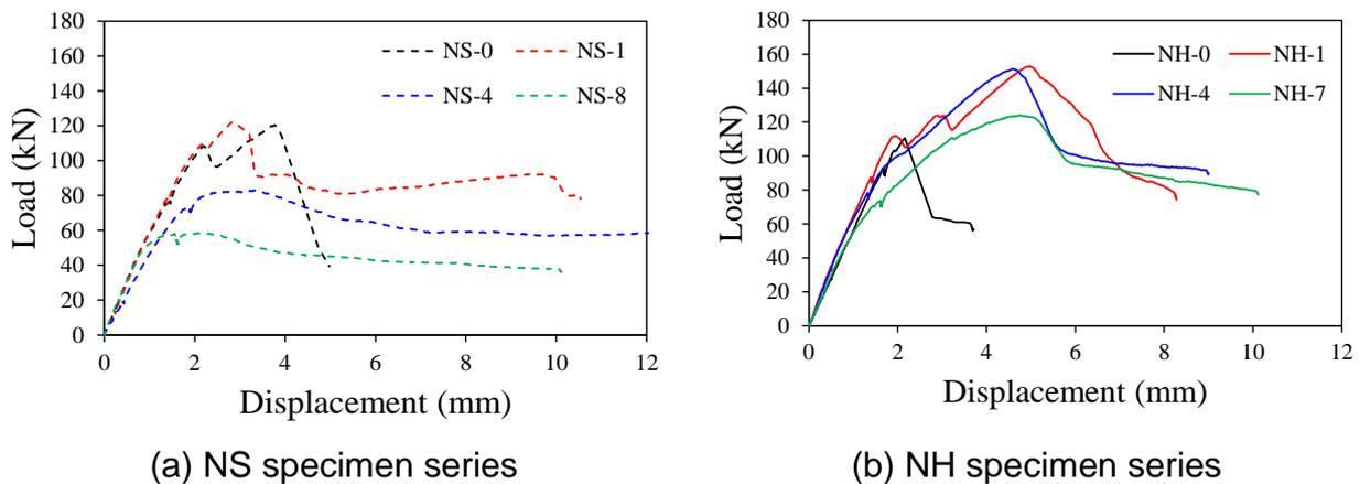
Fig. 4 Comparison of shear behavior according to corrosion rate
